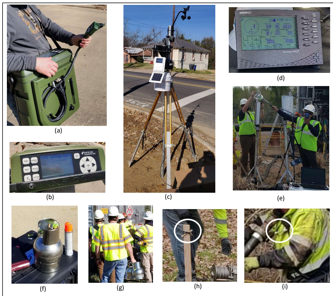
Figure 2: Equipment – Hapsite Unit (a, b), Davis Vantage Pro2 Weather Station (c, d), velocity measurement and canister sample collection from stack at Site 6 (e), air sampling canister (f), duplicate canisters used to sample air inside truck at Site 6 (g), sorbent tube on fixed stake (h), sorbent tube on worker (i)
