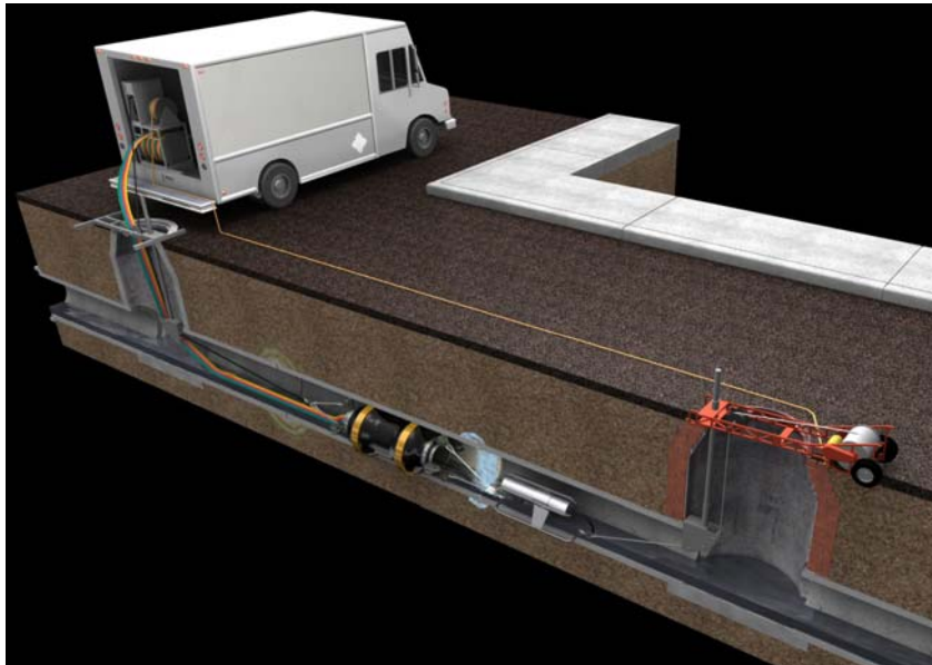
Figure 6. Typical Grout Application Setup
