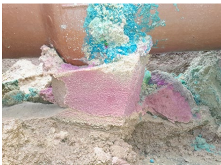
Figure 180: Colored Grout Trial
