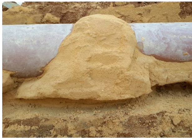
Figure 191: 55 Second Gel Time
