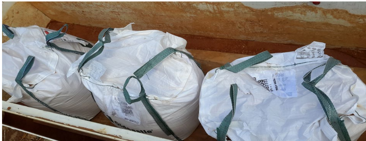
Figure 14: Super Sacks Used to Recreate Typical Soil Loading
