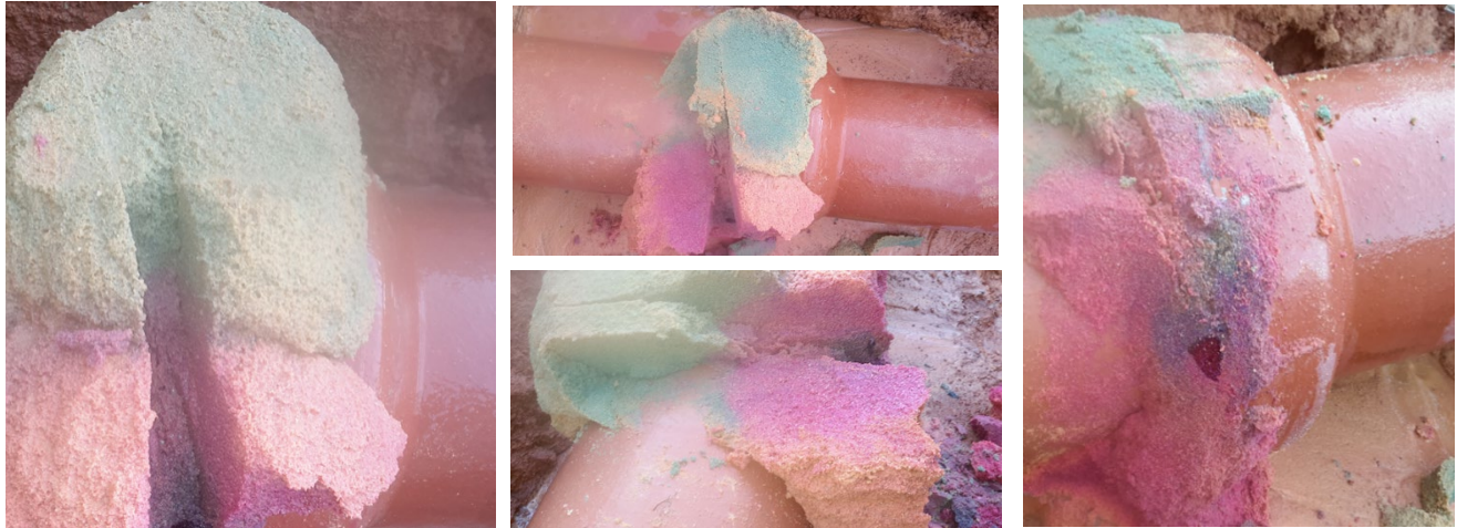
Figures 27, 28, 29, 30: Dissection of Defect A Grout Mass
