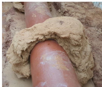
Figure 169: 23 Second Gel Time
