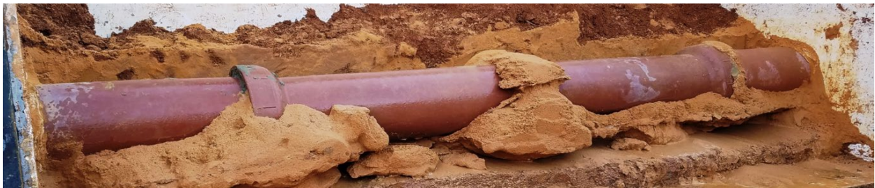
Figure 193: 55 Second Gel Time Grout Formations
