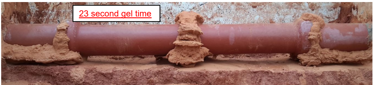
Figure 167: 23 Second Gel Time
