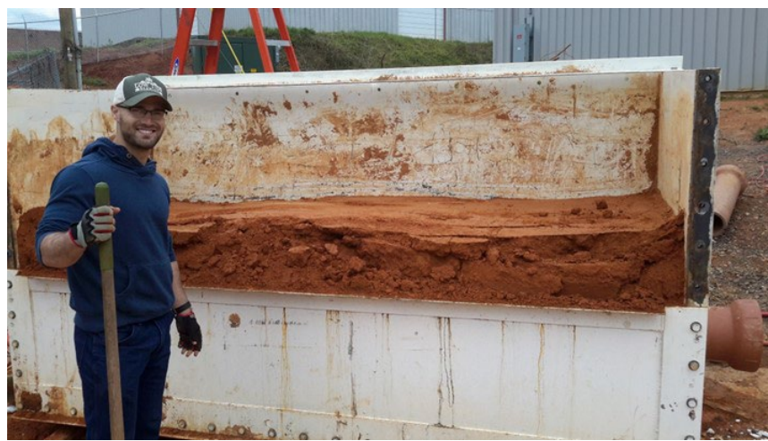
Figure: 90: Disassembly of Grouted Test Cell
