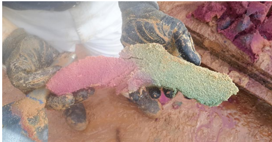
Figure 31: Observation of Distinct Paths of Red and Blue Dyed Grouts
