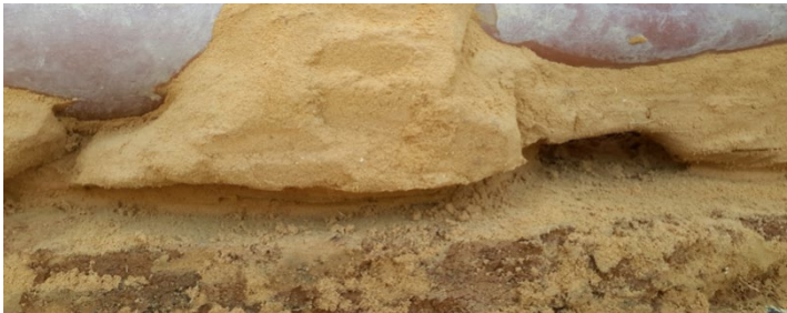
Figure 163: 55 Second Gel Time Pipe Support
