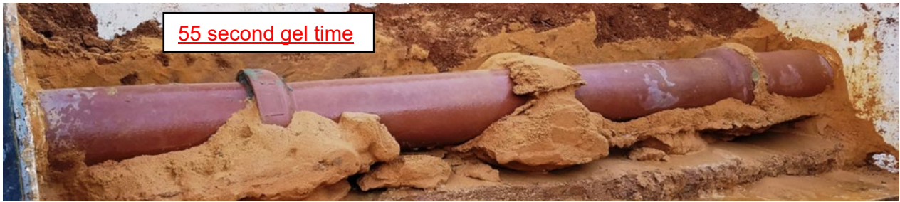
Figure 166: 55 Second Gel Time
