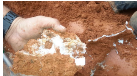
Figure 156: Neat Grout Fin Dissection
