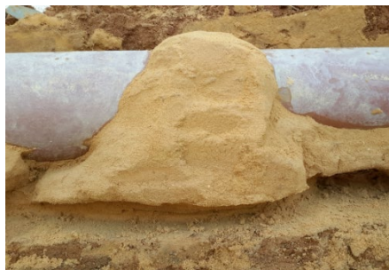
Figure 168: 55 Second Gel Time
