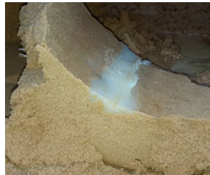
Figure 178: Sand Grout Trial
