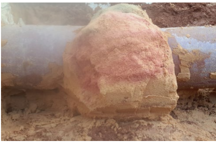
Figure 183: Colored Grout Trial
