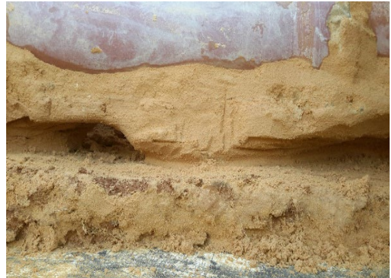
Figure 162: Gel / Soil Matrix at Base of Trench
