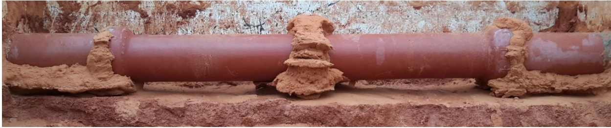
Figure 192: 23 Second Gel Time Grout Formations
