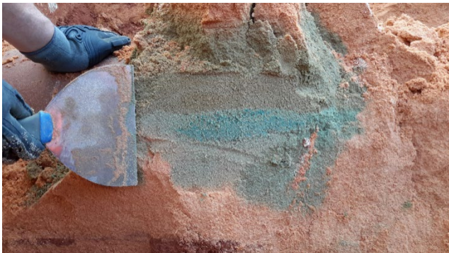
Figure 60: Colored Grout Layers
