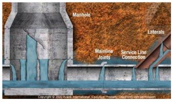
The most common municipal grouting technique uses an inflatable packer to isolate the joint or defect, perform an air test, inject resin if needed and, within a minute, conduct a second air test to validate that the joint has been sealed.
