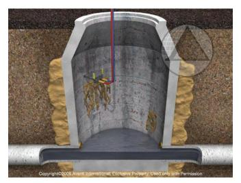
and professor at the Department of Civil and Environmental Engineering at the University of Houston. "Based on its cost-effectiveness, durability and method of leak repair for sewer pipe joints, manholes and laterals, chemical grouting has proven to be the least expensive remediation alternative for stopping leaks and infiltration."
