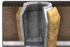
Grout curtain stops infiltration
