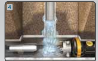
Water infiltration at lateral
