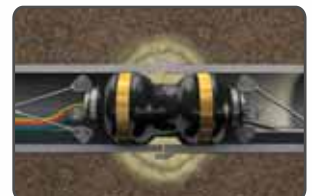
Chemical grout injected into soil
