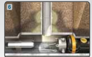
Grout collar stops infiltration
