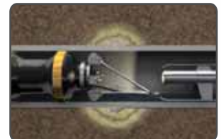
Grout collar stops infiltration
