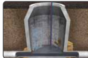
Curtain grouting with wand
