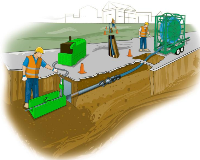
Typical small diameter static pipe bursting operation.
